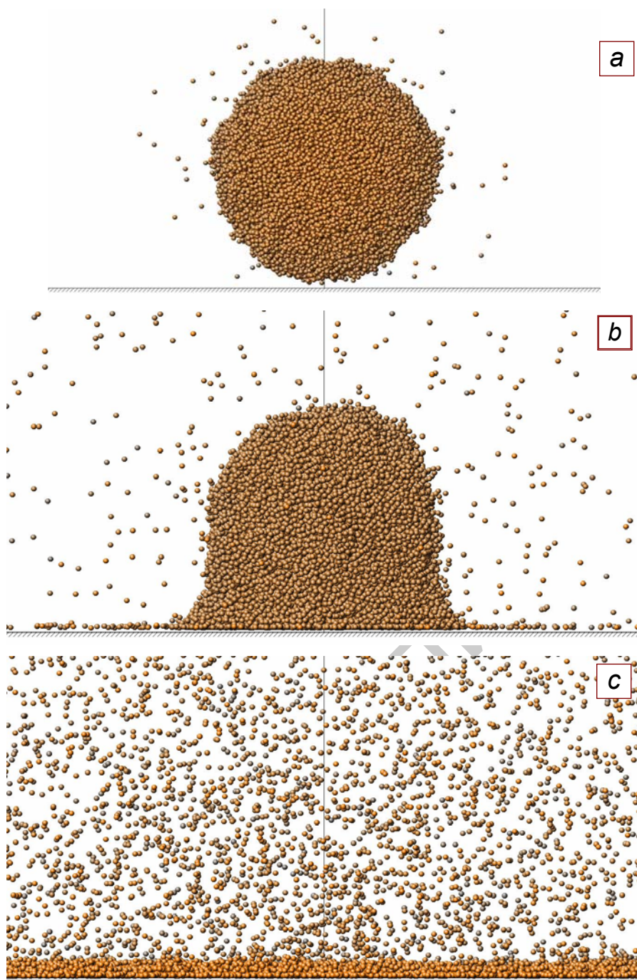
Fig. 1. Snapshots of a droplet consisting of 42000 atoms on the high-energy continual substrate ( \varepsilon_s = 5 , T^* = 0.6 ): (a) lateral view of the initial configuration, (b) intermediate configuration, (c) final (equilibrium) state corresponding to complete wetting.
